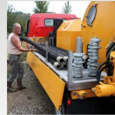
Easy loading and unloading of the 3 m delivery hoses and couplings
