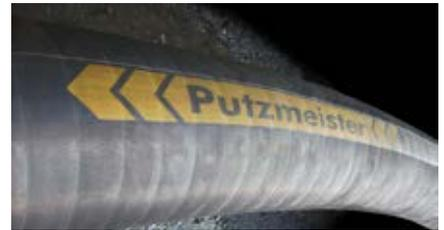
The rotor hose is the only wear part of the pump, and can be replaced very quickly. To protect the hose, it is laid on a fully vulcanised rubber bed.
