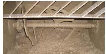
Almost no residual concrete – nearly 100 % of the concrete in the hopper can be delivered to the construction site. Expensive concrete residue disposal is avoided.
