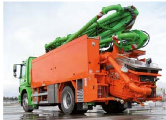
Truck-mounted concrete pump with renovation equipment 20-4 Sanima
